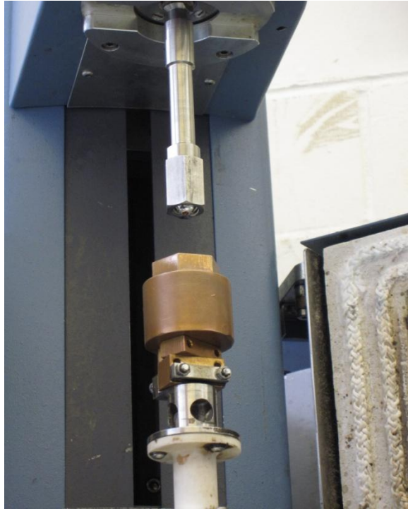
Torque and normal force applied by chuck from top of machine.
