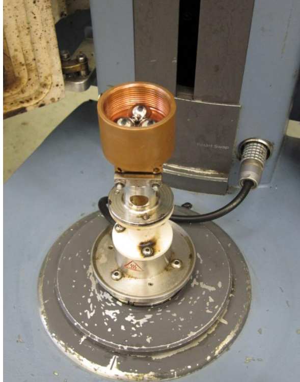
Cup machined for torsion bar geometry in TA DSR.
