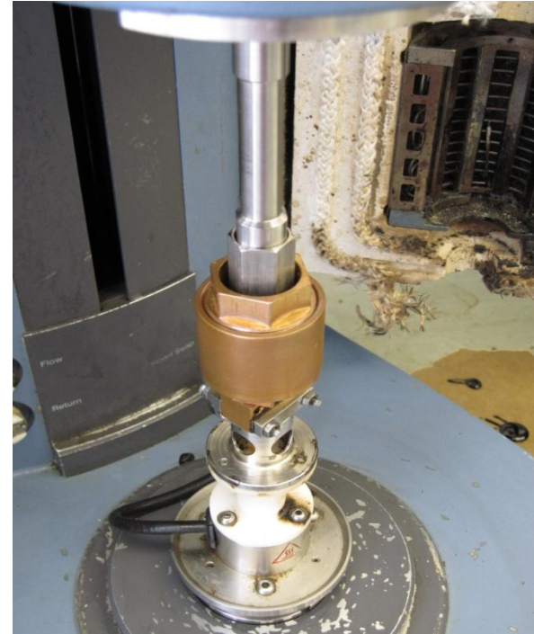
Before testing zero gap is established using cup and chuck.
