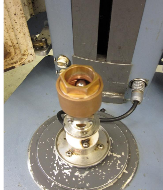
Balls are fixed by lid that screws into cup.
